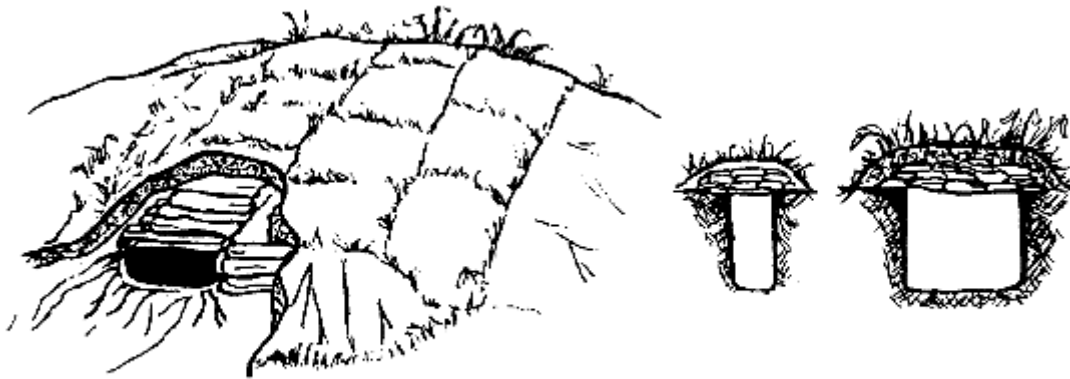
Figure 4-6. Sandbags protected with sod and earth cover.
